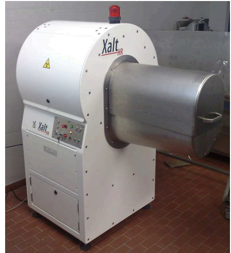
Fig. 1. The Xalt micro-CT scanner at IFC-CNR, Pisa, Italy
