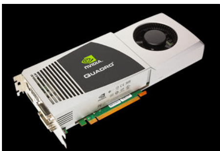
Fig. 1. Nvidia's Quadro FX 5800 comprising 240 thread processors and 4 Gb onboard graphics memory [6].
