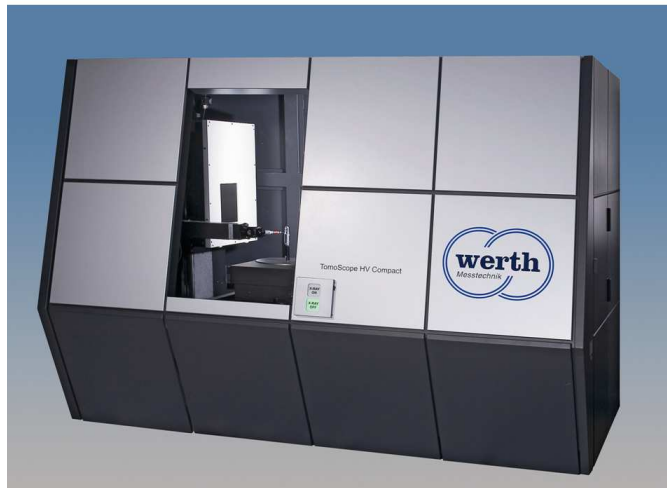
Fig. 1. State–of–the–art dimensional CT scanner used for our studies. The scanner is capable of CT rasterization and of ROI tomography. It acquires in circular and spiral mode.
