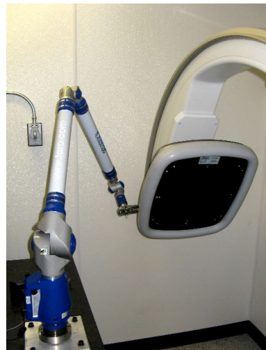
Fig. 2. High accuracy measurements of 3-D geometry with use of FARO-arm.
